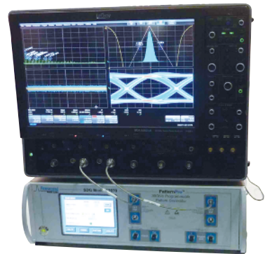
The high-speed Model 12070 (bottom) provides one or two output channels with programmable patterns, data rate, and amp/offset.
