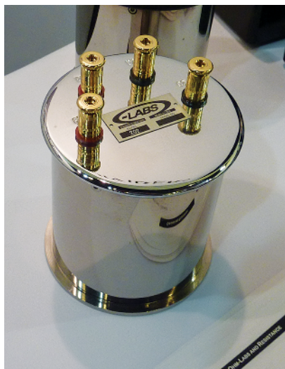
Designed to operate in an oil bath at 25^{\circ}\text{C} for calibrating resistance meters, the Model 202 reference resistor's value changes less than 1 ppm/ ^{\circ}\text{C} .
